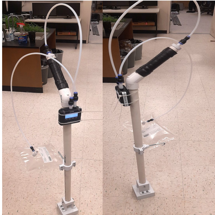
Schematics of the VOCs sampling system
