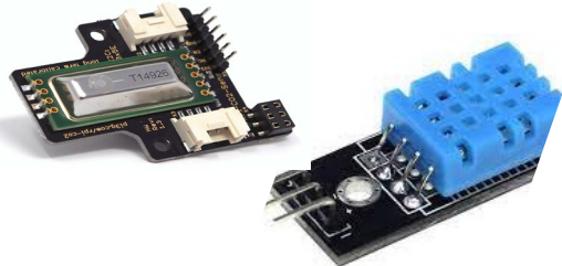
Potential to add temperature, humidity, and CO 2 sensors
